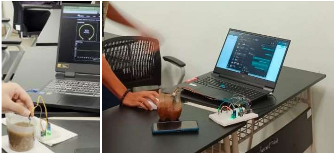
Fig. 1. Demonstration of an IoT project during the DIY IoT workshop using a soil moisture sensor, an ESP32, and an Adafruit IO Dashboard.
