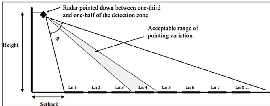
**Figure 5.** Height of device installation (Houston Radar, 2018).
