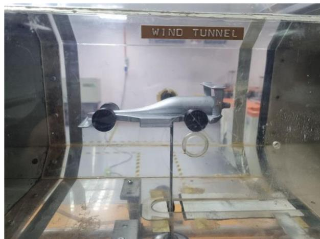
**Figure 7.** Position of F1 in school car model at the centre of Wind tunnel testing section
