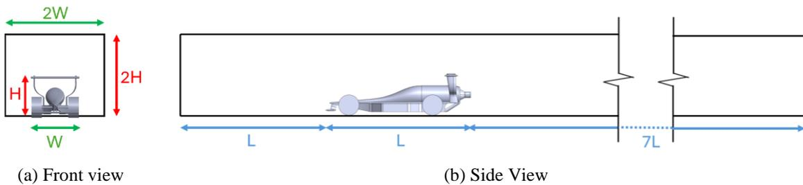
Figure 3. Virtual wind tunnel size
