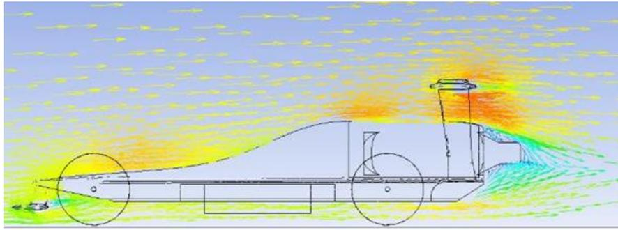
**Figure 14.** F1 in Schools car model 3 side view velocity plot
