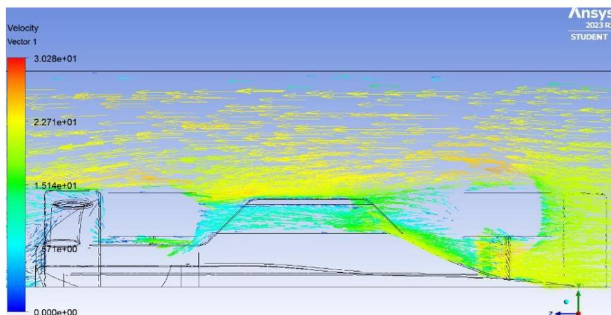
**Figure 13.** F1 in Schools car model 2 top view velocity plot
