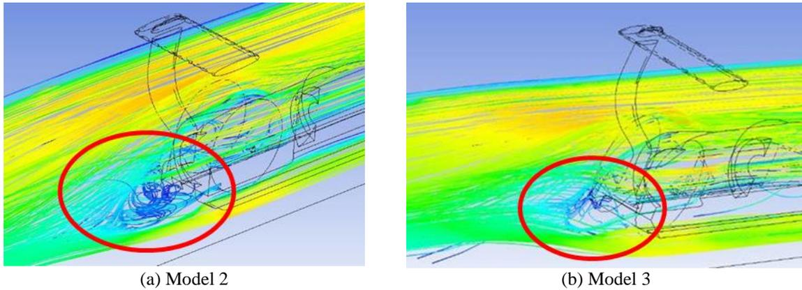
**Figure 15.** Vortex at the rear diffuser
