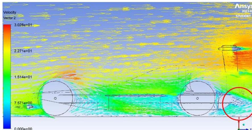
**Figure 12.** F1 in Schools car model 2 side view velocity plot
