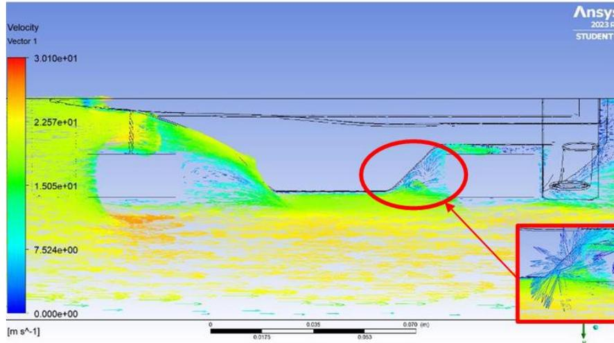
**Figure 11.** F1 in Schools car model 1 top view velocity plot
