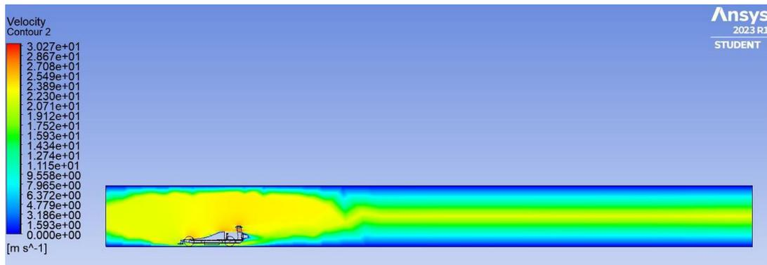
Figure 8. External velocity contour around F1 in Schools car
