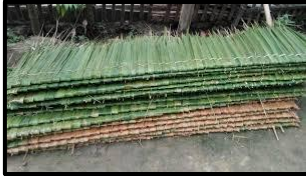
Figure 2.2.4: Nipa Palm Leaves Used to Create Atap Roof
