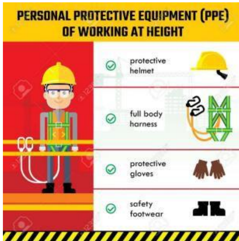
Figure 14 Working at height PPE
