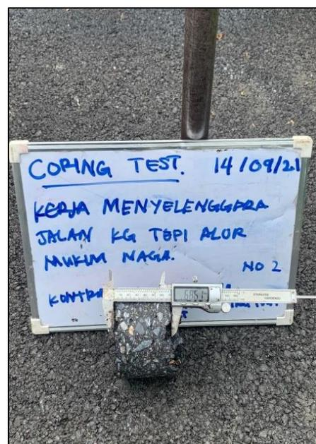
Figure 3.18: Coring Test in Kg Alor Tepi
