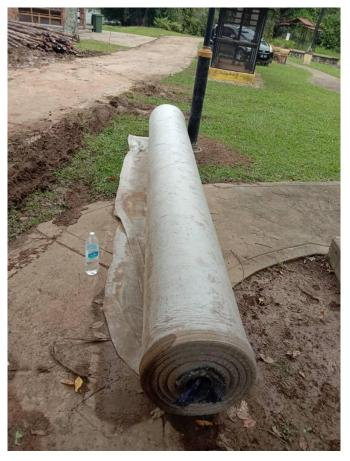
Figure 3.3.5 Non-woven Geotextile Fabric
