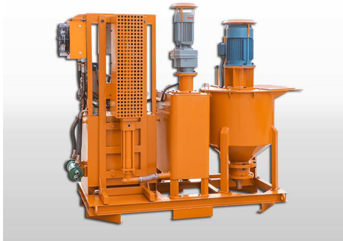
Figure 3.13: 100L Grout mixer for grouting work Source: LEC,2014
