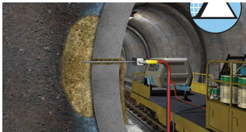
Figure 1.2: Cement grouting for microtunnelling Source: Babcock, 2017
