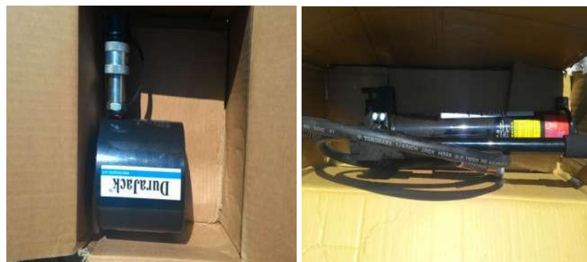
Figure 3.8: Hand jack used for jacking work Source: PDP's document, 2021
