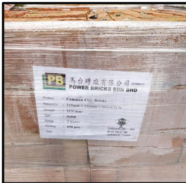
Figure 3. 6 Specification of clay brick
