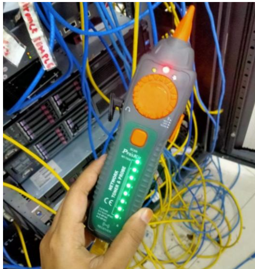
Figure 3.18: Network tower and probe kit
