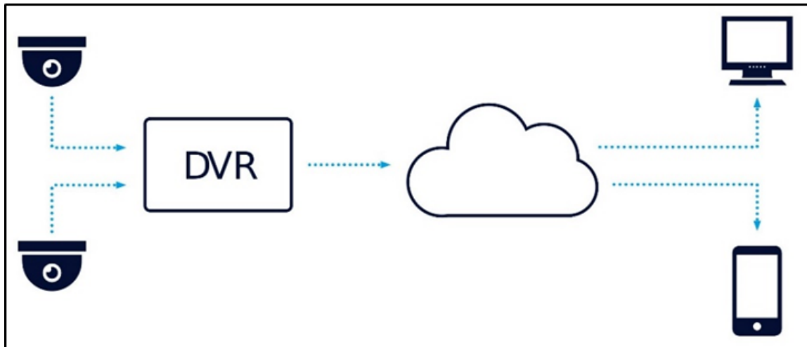
Figure 2.4: How CCTV working
