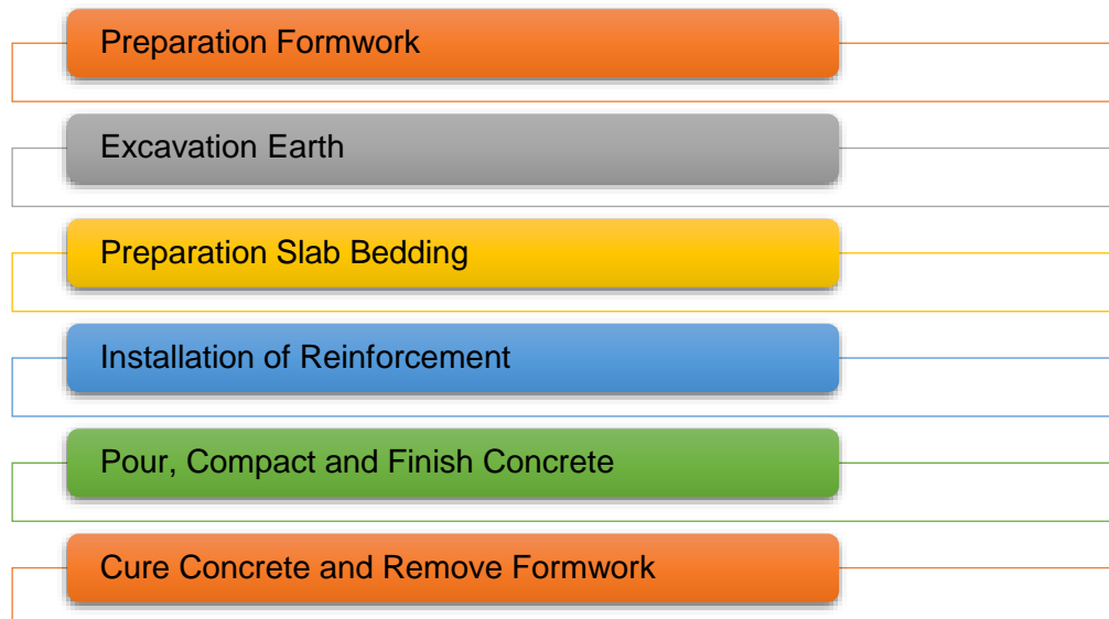
Figure 2.4: The General Construction Process of Floor System
