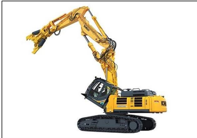
Picture14: Demolish Excavator
