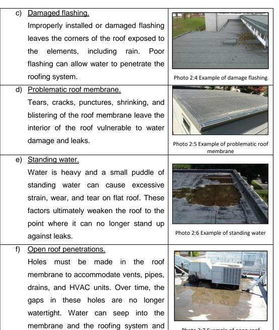
Photo 2:7 Example of open roof penetration
