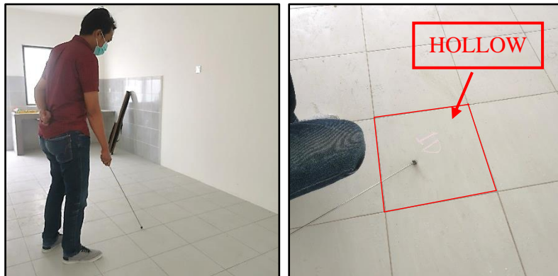
Figure 3.13: Tapping rod is used on the tiles
