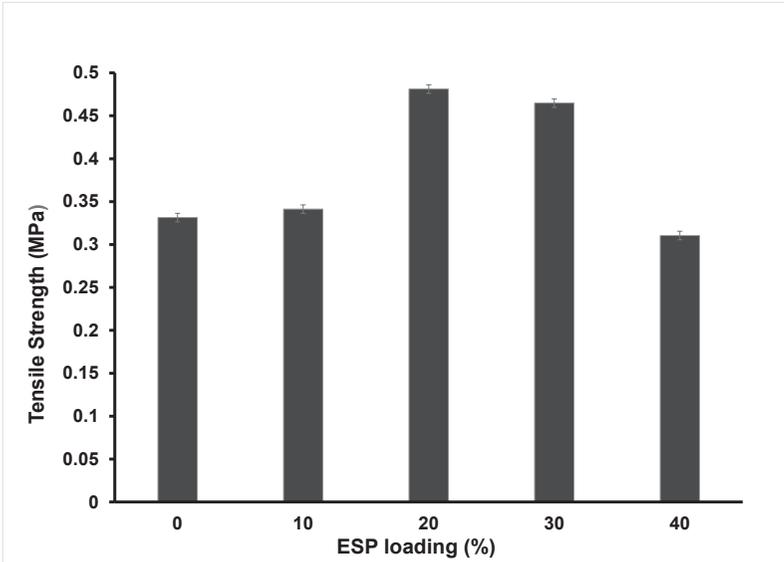
Figure 2: Effect of ESP loadings on the Tensile Strength of PSP bioplastics
