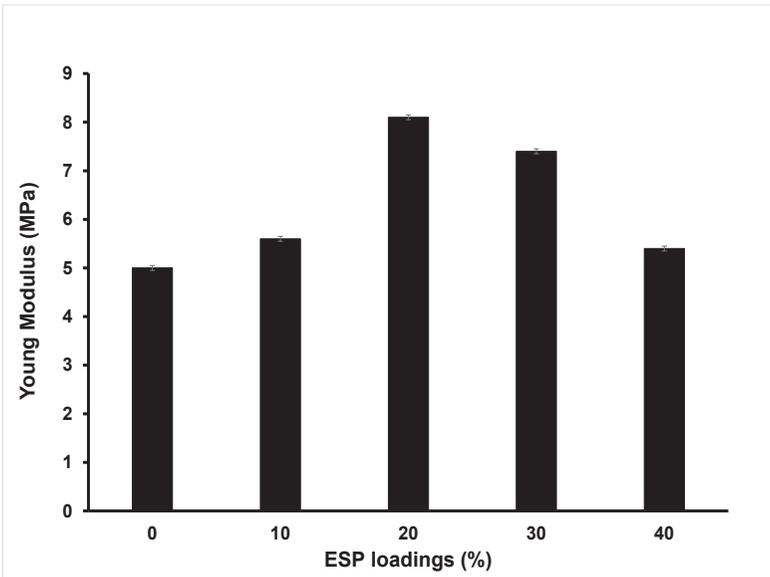
Figure 4: Effect of ESP loadings on the Young's Modulus of PSP bioplastics
