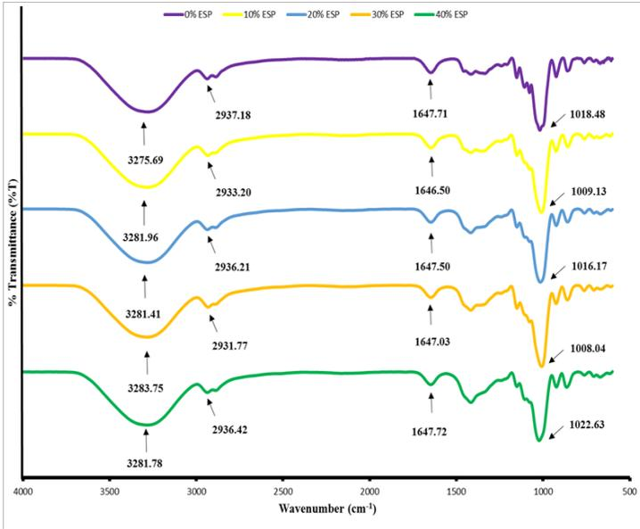
Figure 1: FTIR spectra of PSP/ESP bioplastics
