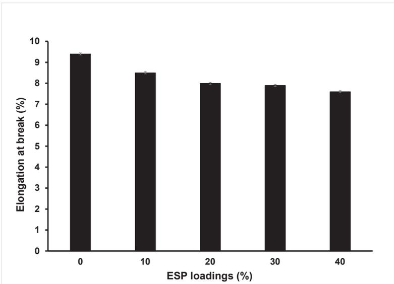
Figure 3: Effect of ESP loadings on the Elongation at Break of PSP bioplastics
