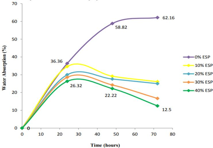
Figure 5: Water Absorption (%) versus Time (hours) of PSP starch bioplastics
