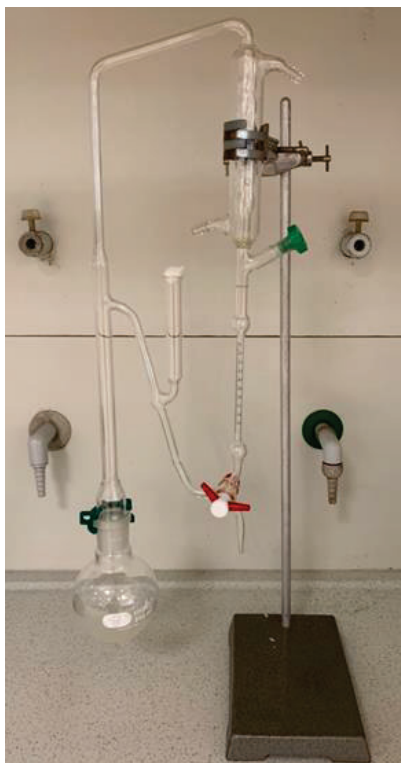
Figure 2: The Clevenger or Dean-Stark apparatus is set for the pharmacy undergraduates for their laboratory practical (left). The dried cloves were mixed with Celite® in a mortar, to make a homogenous powder prior to the distillation (right) (Source: authors' own collection)
