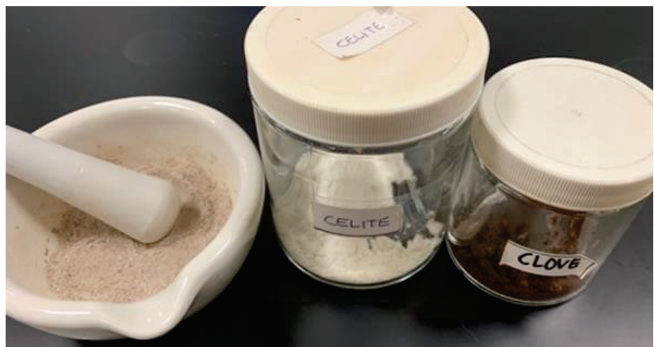
Figure 2: The Clevenger or Dean-Stark apparatus is set for the pharmacy undergraduates for their laboratory practical (left). The dried cloves were mixed with Celite® in a mortar, to make a homogenous powder prior to the distillation (right) (Source: authors' own collection)
