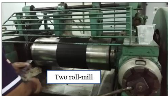
Figure 2: Two-roll mill machine used to prepare XNBR/BRR blends
