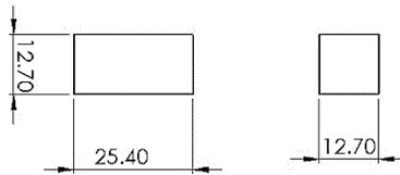
Figure 1: Shape and size of the ASTM D695 specimen in millimeters
