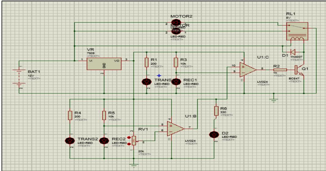
**Figure 2. Schematic Circuits for Smart Auto-Feed Paper Shredder**
