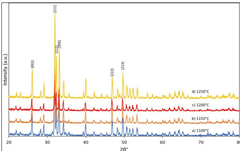
Figure 4: XRD patterns of eggshell-derived HA samples sintered at temperatures ranging from 1100 °C to 1250 °C
