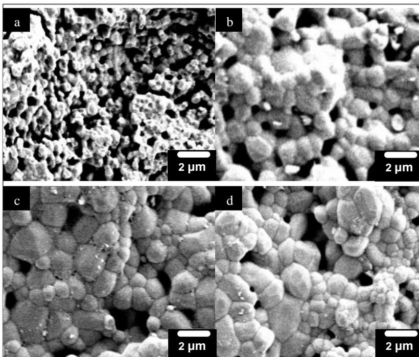
Figure 5: FESEM images of eggshell-derived HA samples sintered at; (a) 1100 °C, (b) 1150 °C, (c) 1200 °C, and (d) 1250 °C
