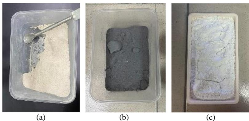
Figure 1: The HA powder preparation: (a) crushed eggshell, (b) eggshell calcined at 700 °C, and (c) ball-milled mixture calcined at 800 °C
