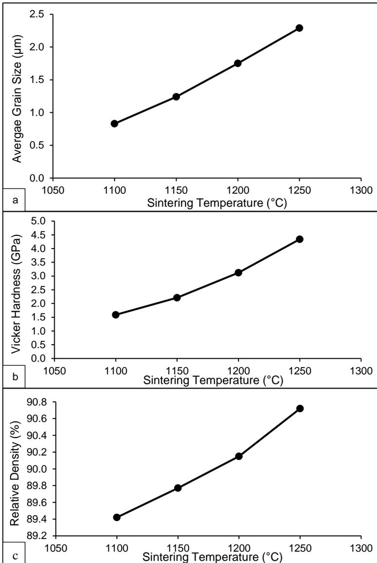
Figure 6: The effect of sintering temperature on; (a) average grain size, (b) Vickers hardness, and (c) relative density of eggshell-derived HA samples
