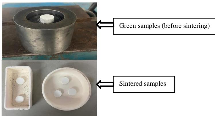
Figure 2: As-prepared dense and sintered eggshell-derived HA samples
