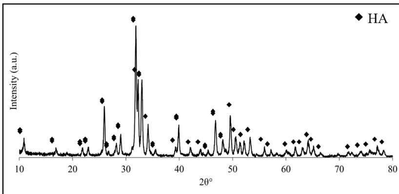
Figure 3: XRD pattern of eggshell-derived HA powder heat treated at 800 °C
