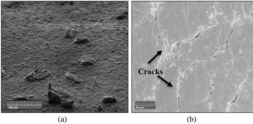
Figure 6: SEM micrograph of; (a) undamaged rubber (500 X magnification), and (b) 100,000 cycles rubber (1000 X magnification)
