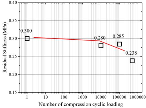
Figure 5: Residual stiffness against number of compression cyclic loading between undamaged and damaged specimens
