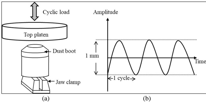
Figure 3: (a) Schematic of uniaxial cyclic compressive tests, and (b) constant amplitude-controlled loading method used in this study
