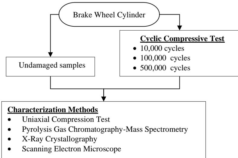
Figure 2: Process flow chart showing the applied characterization route of samples
