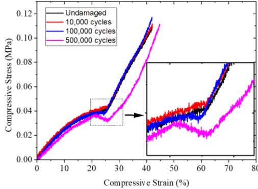
Figure 4: Typical compressive stress-strain curves of rubbers after compressive cyclic loading
