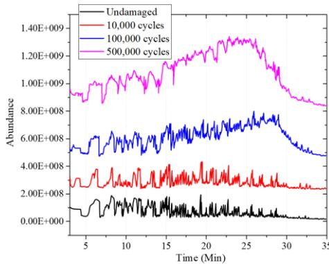
Figure 8: GC-MS comparison between undamaged and damaged rubber
