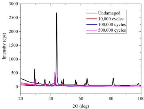
Figure 7: XRD pattern between undamaged and damaged samples under cyclic loadings
