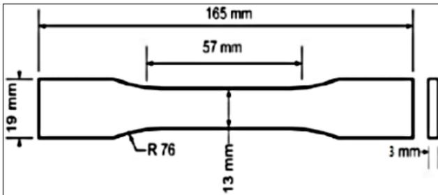
Figure 1: ASTM D638-Type I standard dimension
