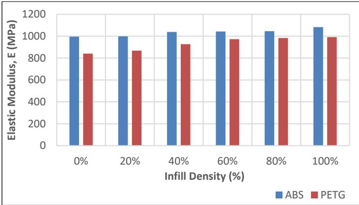
Figure 7: Comparison of Young's modulus at different ABS and PETG infill density
