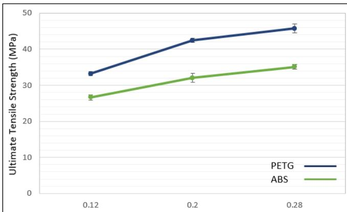
Figure 12: Comparison of layer height effect on the ultimate tensile strength of ABS and PETG materials
