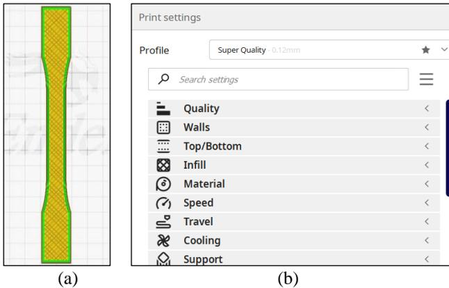
Figure 3: (a) The slicing result of the ASTM D638-Type I model; and (b) print settings options in Ultimaker Cura
