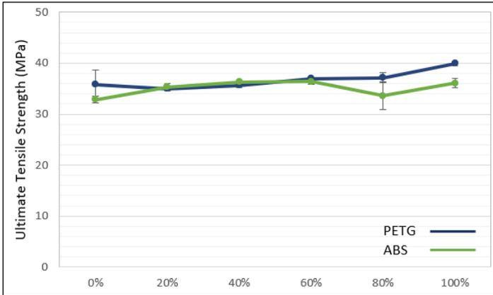
Figure 8: Comparison of ultimate tensile strength at different ABS and PETG infill density
