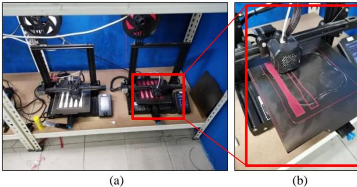
Figure 4: (a) Ender 3 printer units; and (b) specimen being printed on the heating bed
