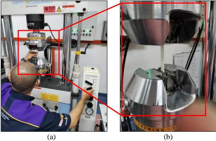
Figure 6: (a) Tensile test was done using Universal Tensile Testing machine model Servopulser Shimadzu; and (b) each end of the specimen were attached on the testing machine machine
