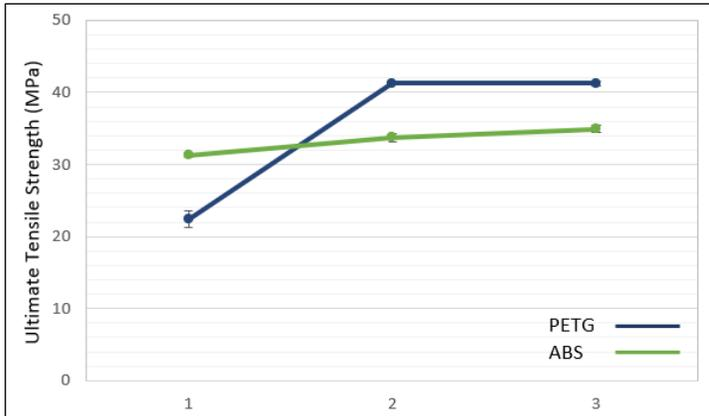
Figure 10: Comparison of wall perimeter effect on ultimate tensile strength of ABS and PETG materials
