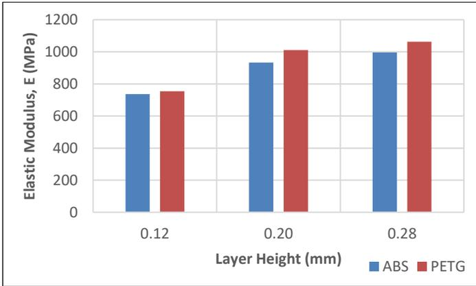
Figure 11: Comparison of layer height effect on the Young's modulus of ABS and PETG materials
