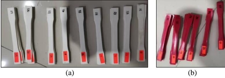
Figure 5: (a) Specimen for ABS material; and (b) specimen for PETG material
