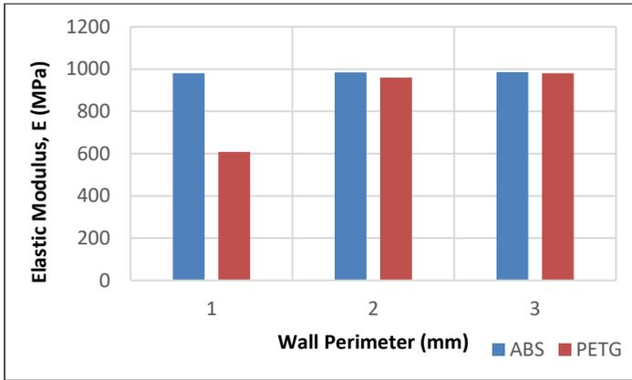
Figure 9: Comparison of wall perimeter effect on Young's modulus of ABS and PETG materials
