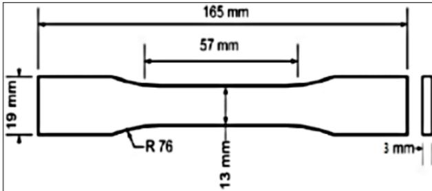
Figure 1: ASTM D638-Type I standard dimension
