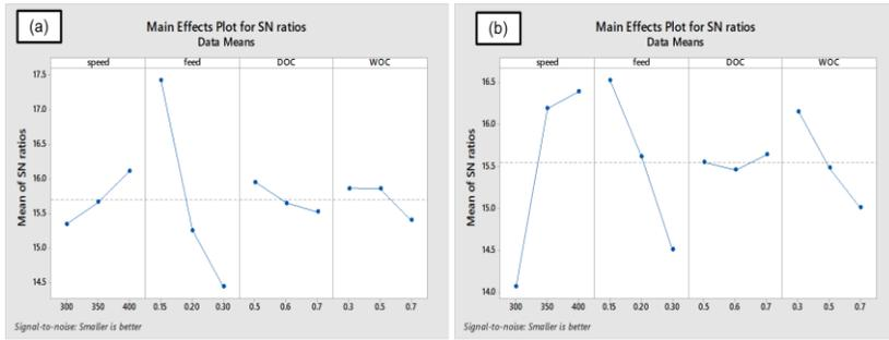
Figure 2 Main effect plot for SR in; (a) MQL condition, and (b) cryogenic conditions
