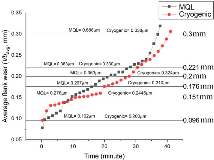
Figure 6: Comparison of average flank wear when cutting AISI 4340 in MQL and cryogenic conditions using experiment 8 for  $V_c= 400$  m/min,  $f_z= 0.2$  mm/tooth, DOC= 0.5 mm and WOC= 0.7 mm
