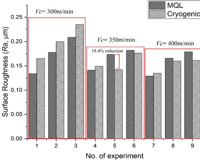
Figure 3: SR experimental results for various cutting parameters when cutting under MQL and cryogenic conditions
