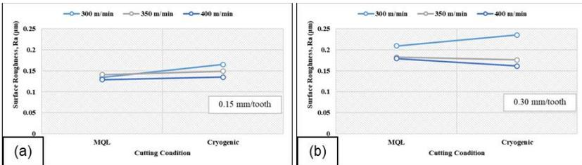
Figure 5: Effect of cooling/lubricating on SR at different cutting speeds with constant feed rate; (a) 0.15 mm/tooth, and (b) 0.3 mm/tooth
