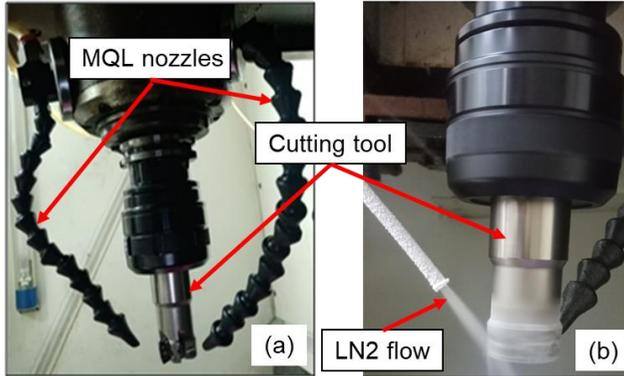
Figure 1: Experimental setup for; (a) MQL, and (b) cryogenic
