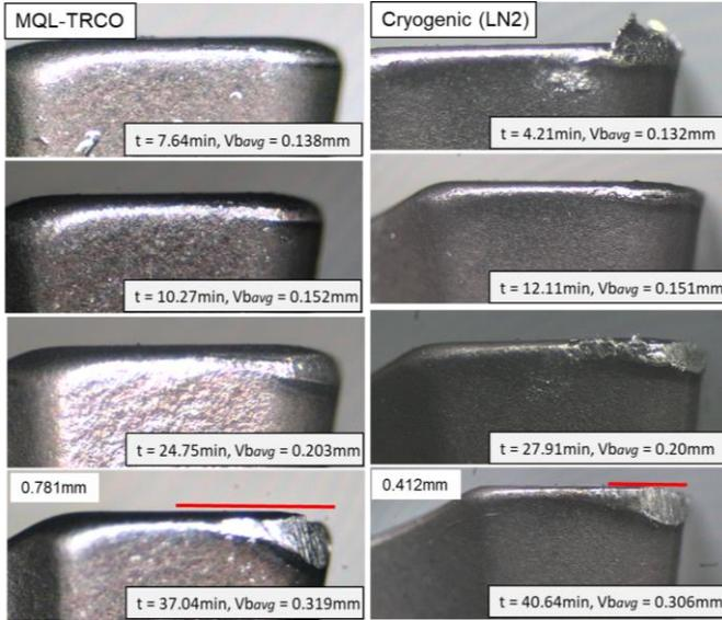
Figure 7: Progressive tool wear of AISI 4340 when cutting in MQL and cryogenic condition using experiment 8 for  $V_c= 400$  m/min,  $f_z= 0.2$  mm/tooth, DOC= 0.5 mm and WOC= 0.7 mm
