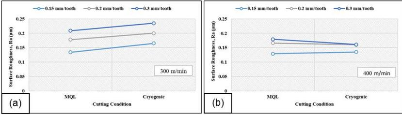
Figure 4: Effect of cooling/lubricating on SR at different feed rates with constant cutting speed; (a) 300 m/min, and (b) 400 m/min
