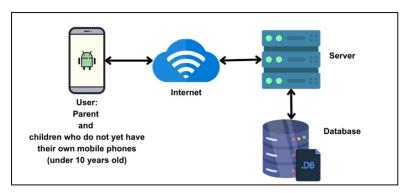
Figure 1: Logical Diagram of Child-CyberCare Mobile Application
