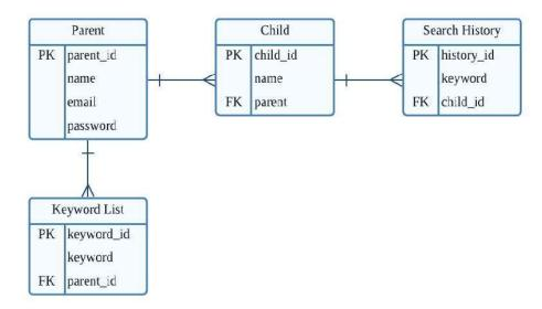
Figure 3: Entity Relationship Diagram of Child-CyberCare Mobile Application
