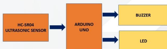
Figure 1.2: Block Diagram of Child Safety Car Reverse Parking System
