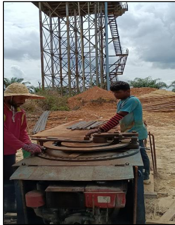
Figure 3.2: Bar bender machine
