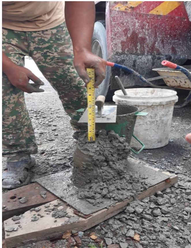
Figure 3.7.2: Slump test result
