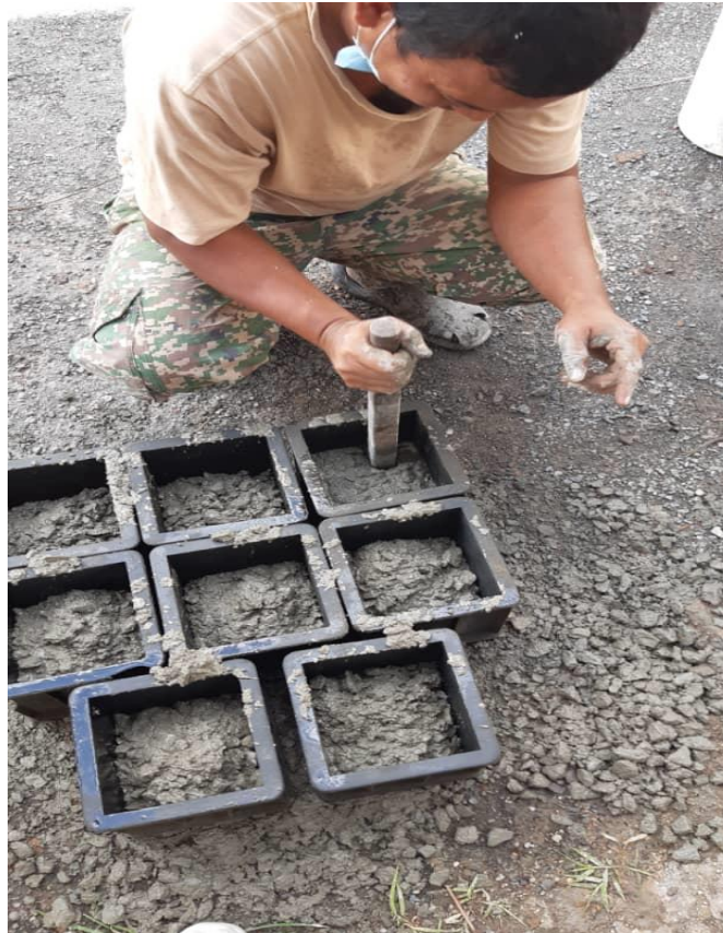
Figure 3.7.3: Workers fill in the concrete in the cube mould
