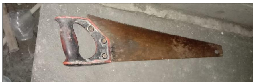
Figure 3.6: Hand saw that are used to cut the plywood.
