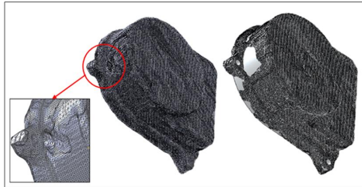
Figure 6: Extruded boss on the curved surface of scanned model to cover up the defects.
