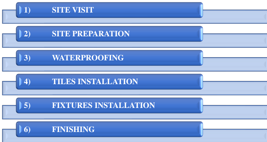
Figure 3.3: Method Statement of Toilet Renovation.
