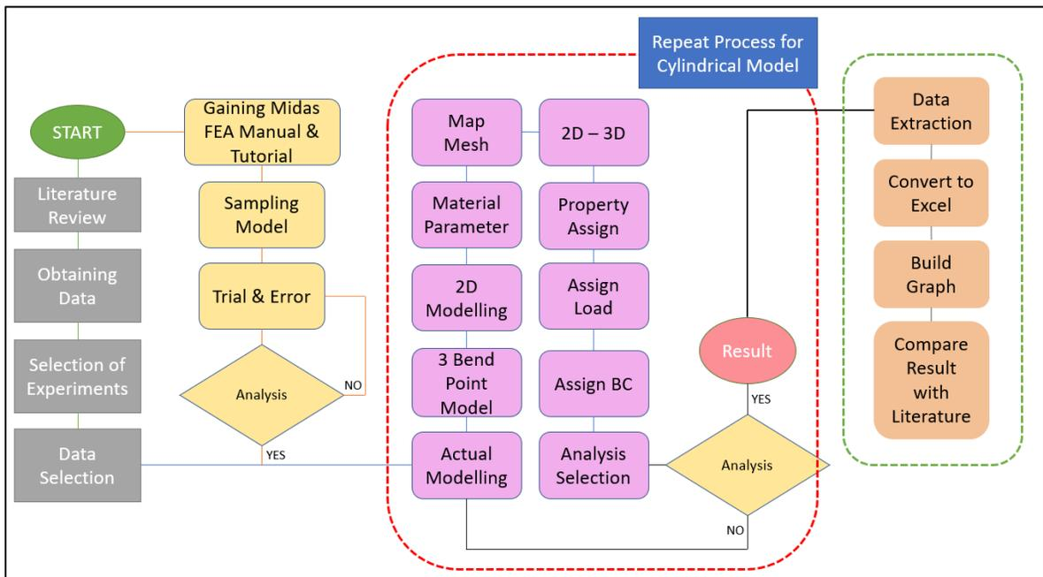
**Figure 3.** Process Flow
