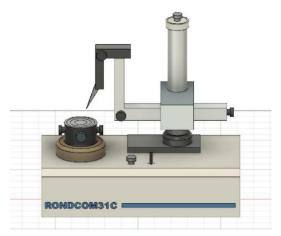
Figure 2. Model of roundness measuring machine
