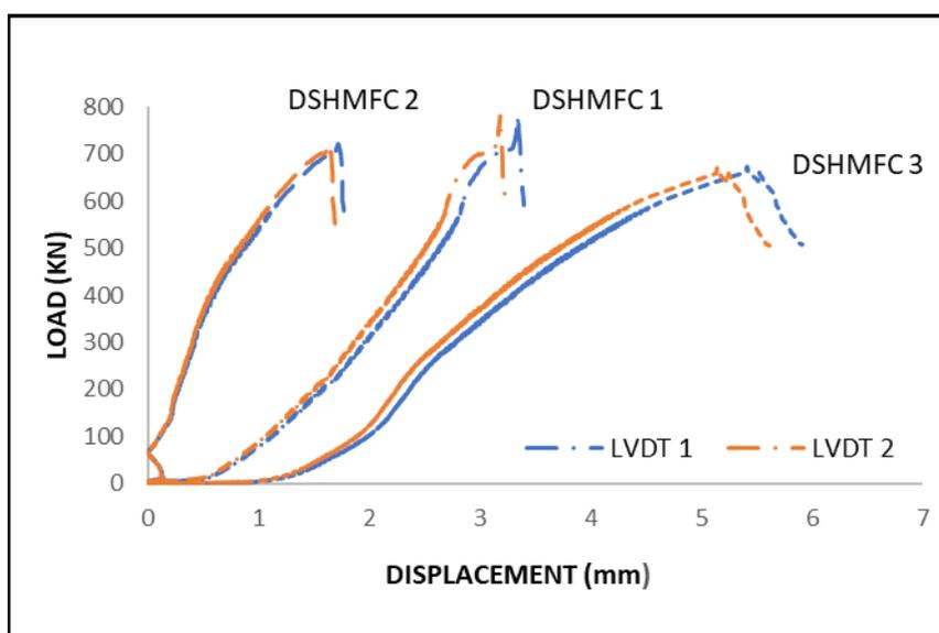
**Figure 4.** Axial load-displacement for DSHMFC specimens.
