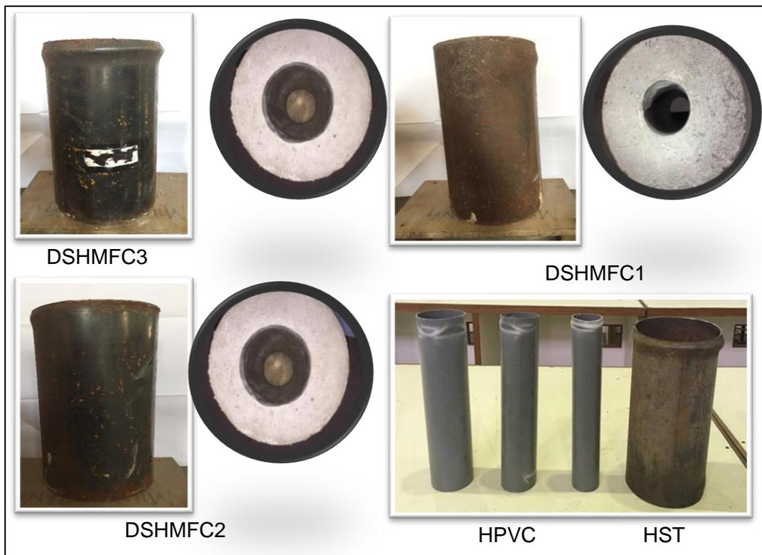
**Figure 5.** Failure mechanisms in DSHMFC specimens.
