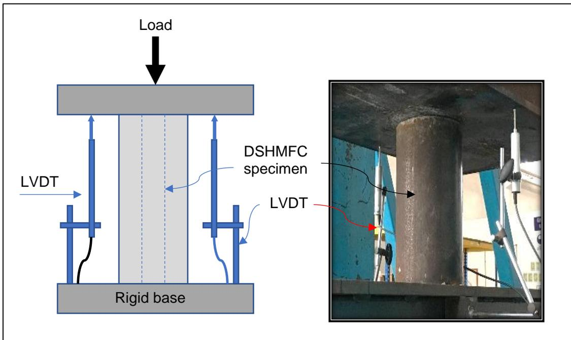
**Figure 3.** Compression test setup and instrumentations of DSHMFC specimens.
