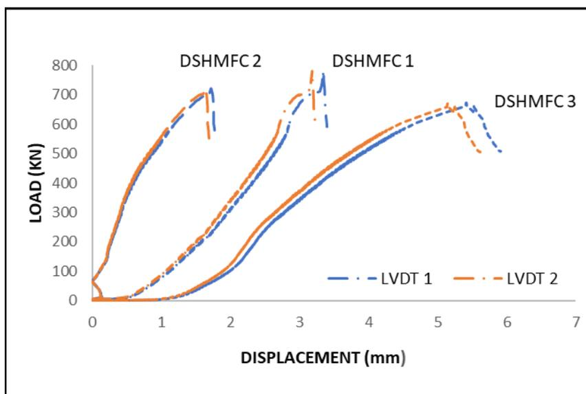
**Figure 4.** Axial load-displacement for DSHMFC specimens.
