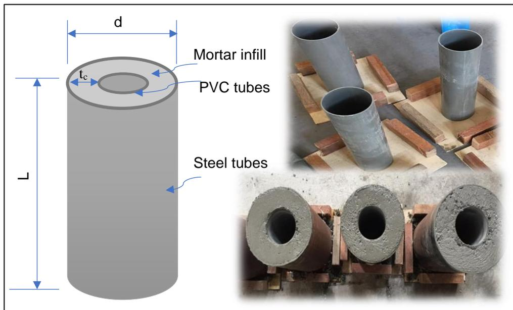
**Figure 2.** Double skin hollow mortar-filled columns (DSHMFC) sample preparations.
