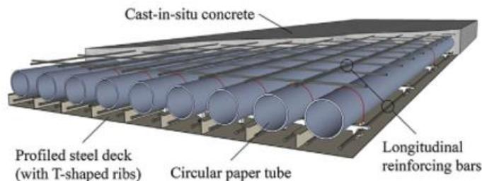
Figure 1: Tube-Deck Slab System Illustration [13]
