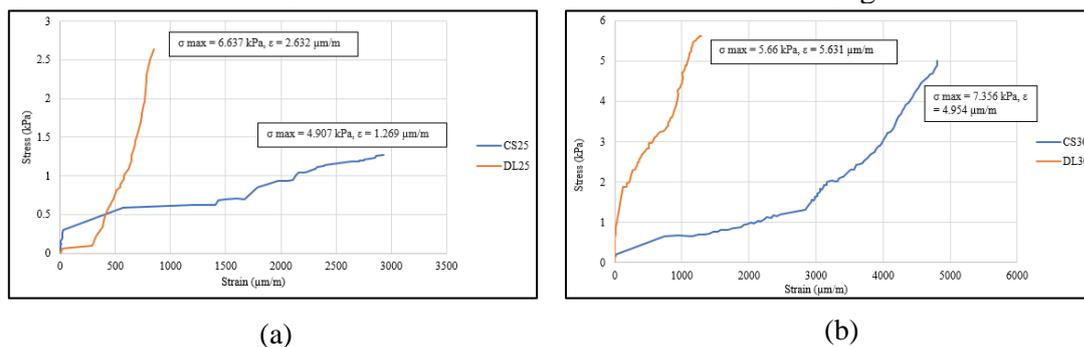
Figure 8: Stress-Strain Behaviour (a) C25; (b) C30.
