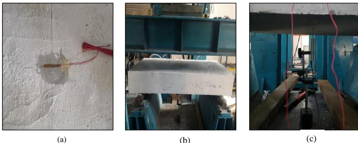
Figure 5: Testing of Slab (a) Strain Gauge on Slab Surface; (b) Slab on Support of Reaction Frame; (c) Installation of LVDT Under the Slab Specimen.
