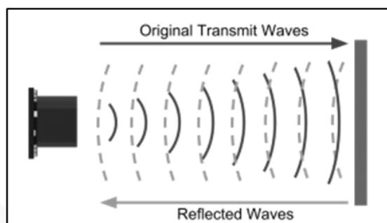
**Picture 1** - High-frequency sound waves reflect from boundaries to produce distinct echo patterns.
