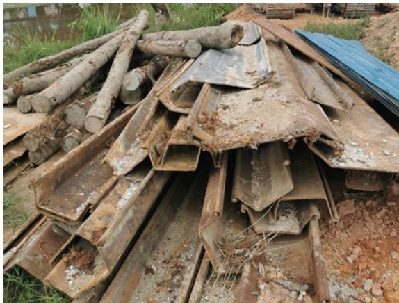
Figure 3.9: Sheet pile of Z-Type (Z) and U-Type (U).
