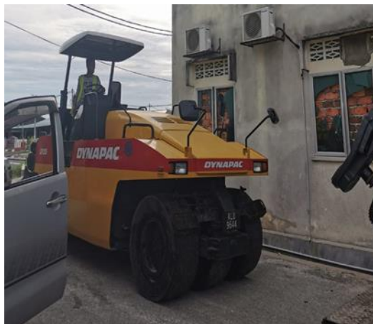
Figure 3.6: Pneumatic tyred roller to compacting uniform coarse soils and rocks.
