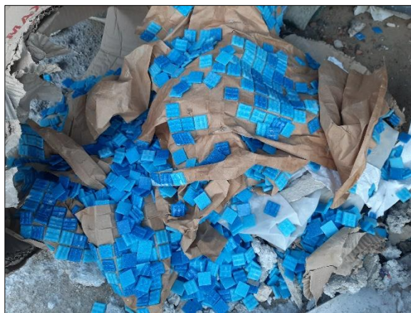
Figure 3.34: damaged of paper-face mosaic tile
