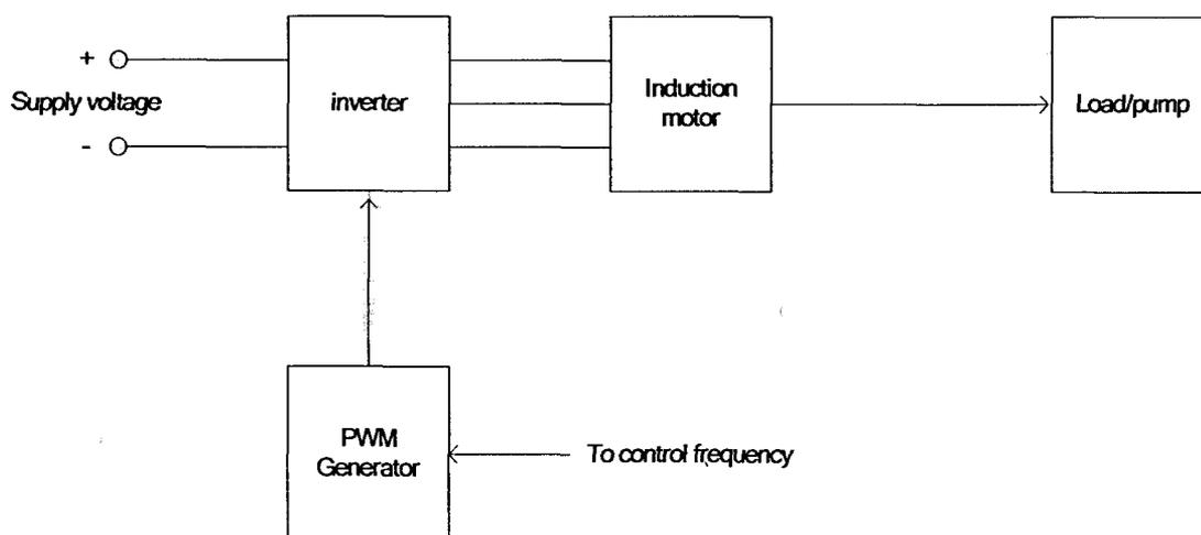
Figure 1.1: Block diagram for simulation model.
