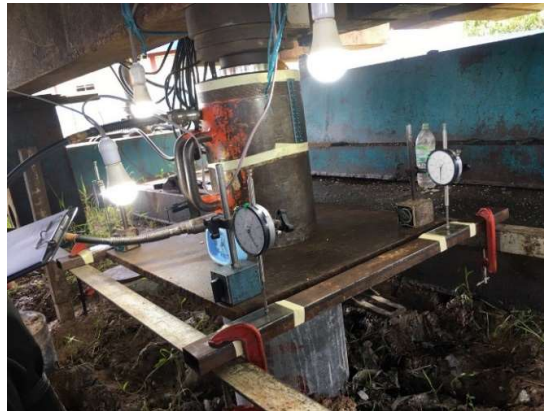
Figure 3.12: Setup for dial gauge and mechanical hydraulic pump
