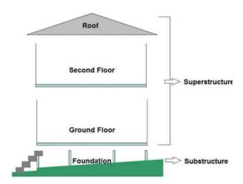
Figure 1.1 Superstructure and Substructure in a Building
