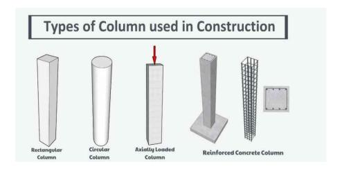
Figure 1.3 Types of Column used in Construction (https://civiconcepts.com/blog/types-of-column)
