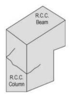
Figure 3.12 Horizontal Crack
