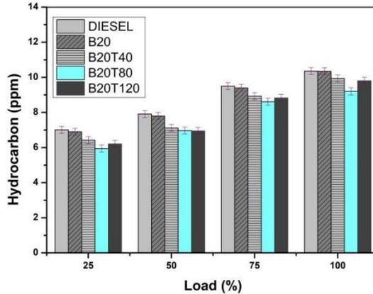
Figure 10: The variation of HC emissions vs. concerning load (%)
