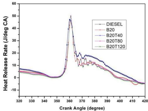
Figure 6: Heat release rate vs. crank angle (degree)
