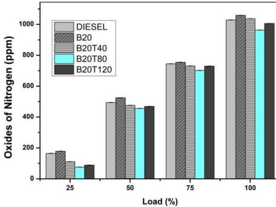
Figure 11: The variation of NOx emissions vs. concerning load (%)
