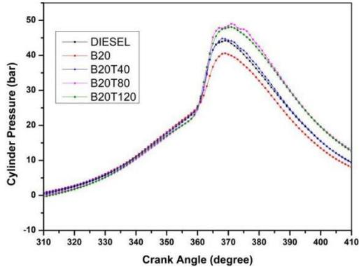
Figure 5: Cylinder pressure vs. crank angle (degree)
