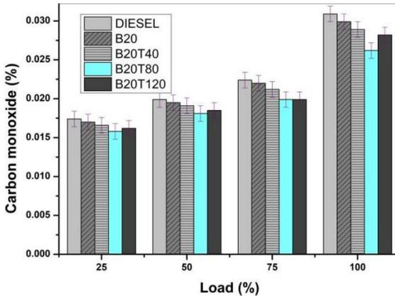
Figure 9: The variation of CO emissions vs. load (%)
