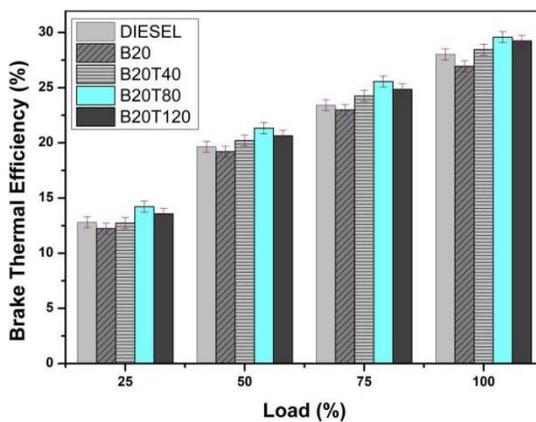
Figure 7: Variation of BTE for various samples concerning various loads
