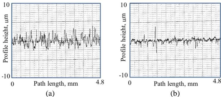
Figure 2: Roughness line profiles for mild steel surface substrate; (a) original, and (b) pre-treated with sulfuric acid at 60 seconds of immersion
