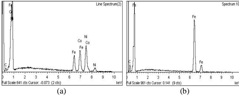
Figure 8: EDS spectrum; (a) Co-Ni-Fe coating, and (b) metal base
