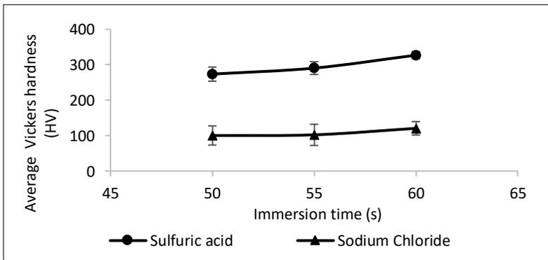
Figure 9: Surface hardness of coated mild steel pre-treated with multiple pickling solutions
