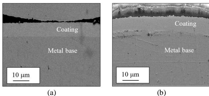
Figure 7: SEM cross-section images coated mild steel ring pre-treated with; (a) sulfuric acid, and (b) sodium chloride at 60 s time immersion
