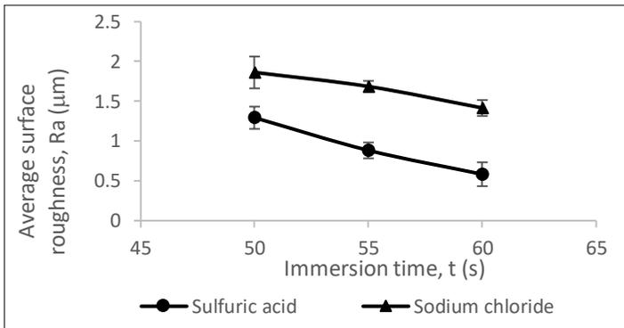
Figure 3: Surface roughness of surface coating pre-treated with different pickling solutions
