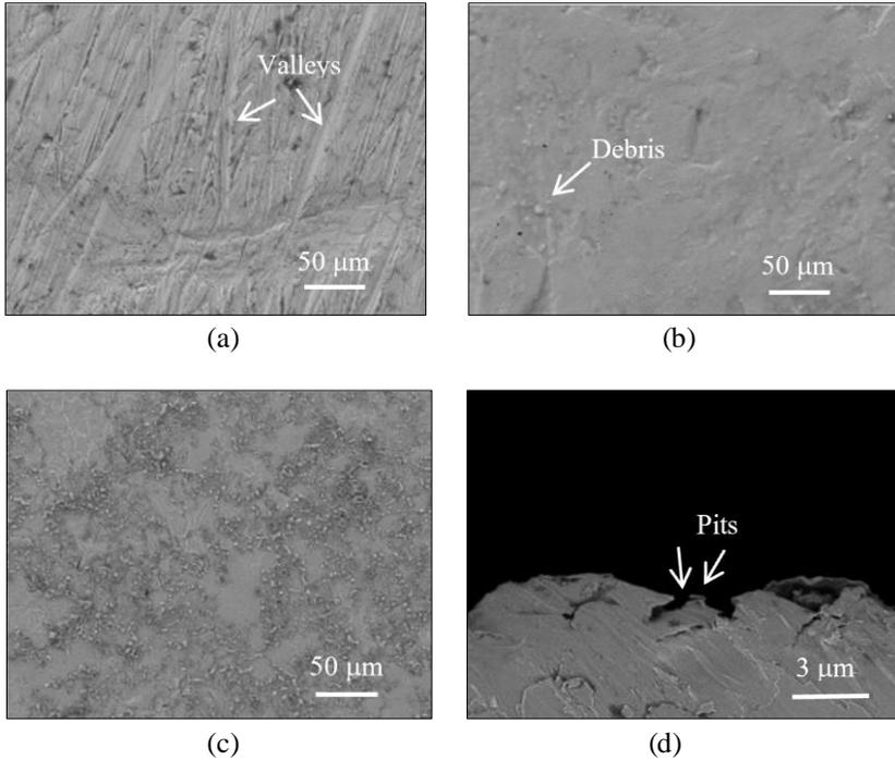
Figure 4: SEM images; (a) original mild steel, (b) mild steel pre-treated with sulfuric acid at 60 s, (c) mild steel pre-treated with sodium chloride at 60 s, and (d) cross-section of mild steel pre-treated with sodium chloride at 60 s
