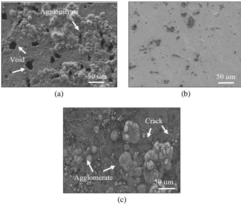
Figure 6: SEM images; (a) coating without pre-treatment, (b) coating pre-treated with sulfuric acid at 60 s, and (c) coating pre-treated with sodium chloride at 60 s
