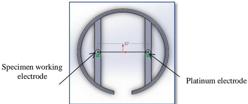
Figure 1: Schematic diagram of electrodes holder in electroplating process (top view)
