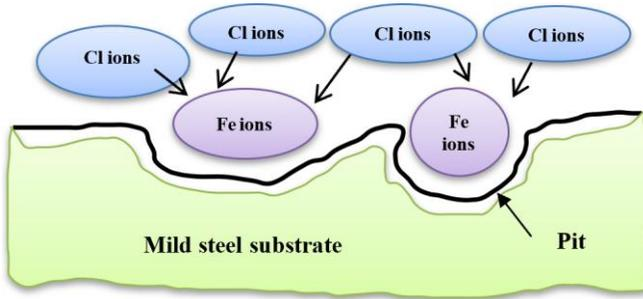
Figure 5: Illustration of sodium chloride reacted with mild steel substrate
