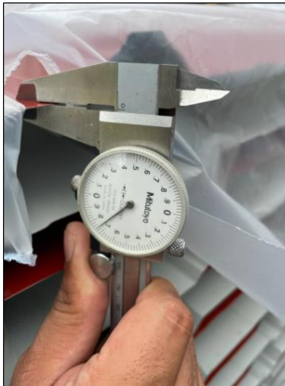
Figure 3.10: Checking the thickness of roofing sheet by using Vernier caliper
