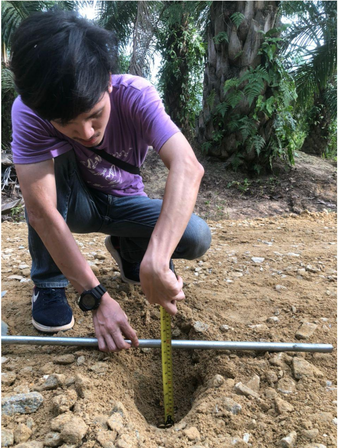
Figure: coring test on Kampung Jawa main road
