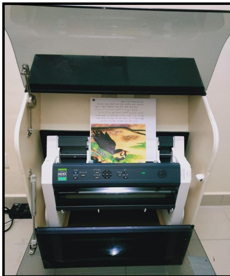
Figure 80: Way to insert braille paper in braille machine
