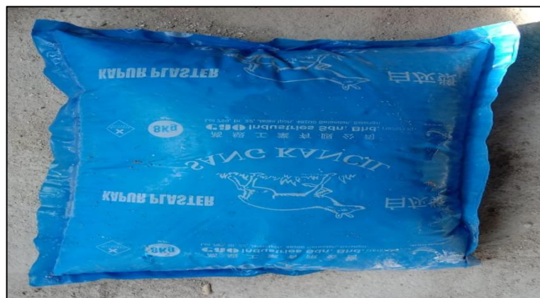
Figure 3.2: The lime used in the plastering work.
