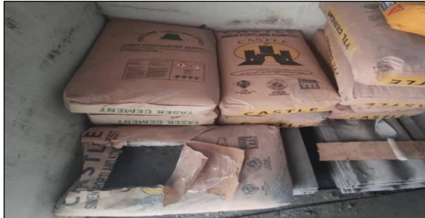
Figure 3.3: The cement used in the plastering work.
