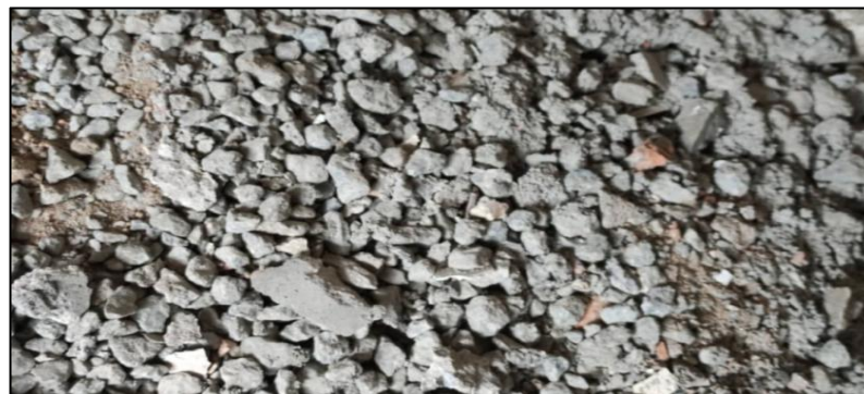
Figure 3.6: Gravel used in concrete.
