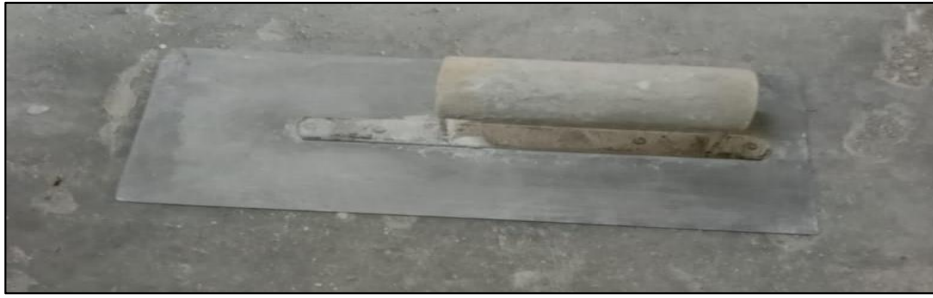
Figure 3.10: Finishing trowel used in the plastering work.
