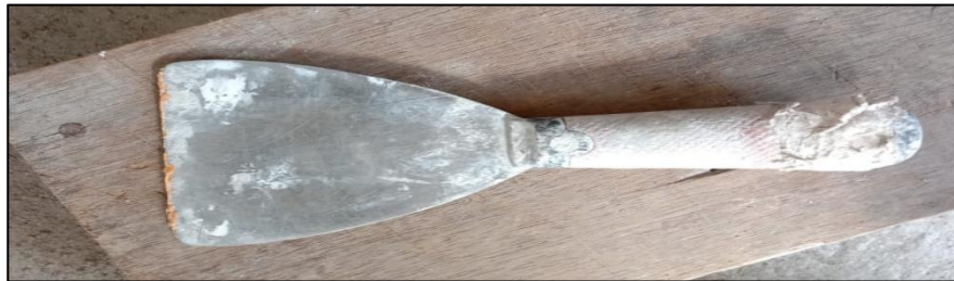
Figure 3.11: Scraper used in the plastering work
