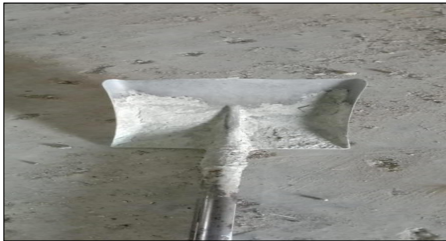
Figure 3.7: Shovel used in the plastering work.
