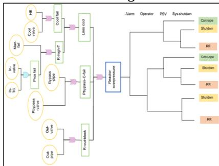
**Bayesian network of reactor overpressure with three-time slices**
