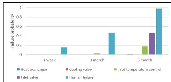
**Failure probability graph of the safety barriers for three time-slices**
