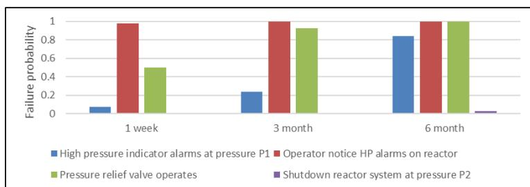
**Conventional risk analysis of reactor overpressure of the ammonia reactor for comparison study**
