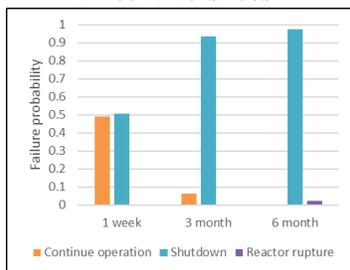
**Failure probability graph of the loss of cooling for three time-slices**
