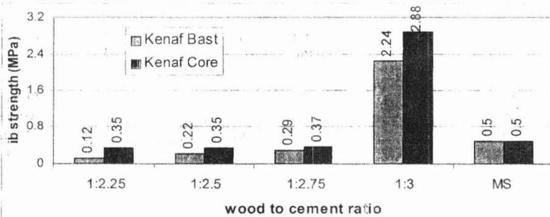
Figure 3: ib values of kenaf based cement bonded particleboard
