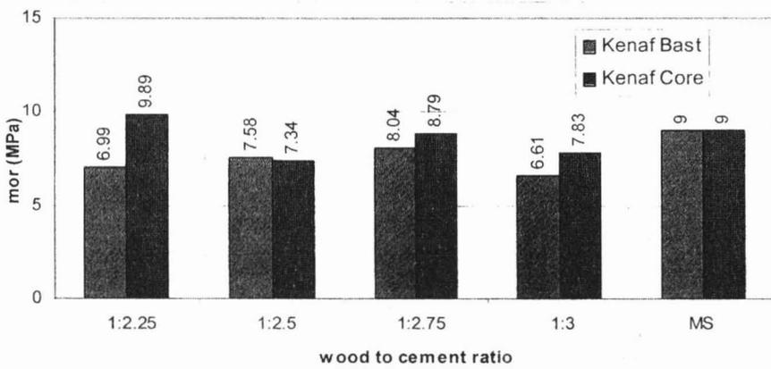
Figure 1: mor values of kenaf based cement bonded particleboard
