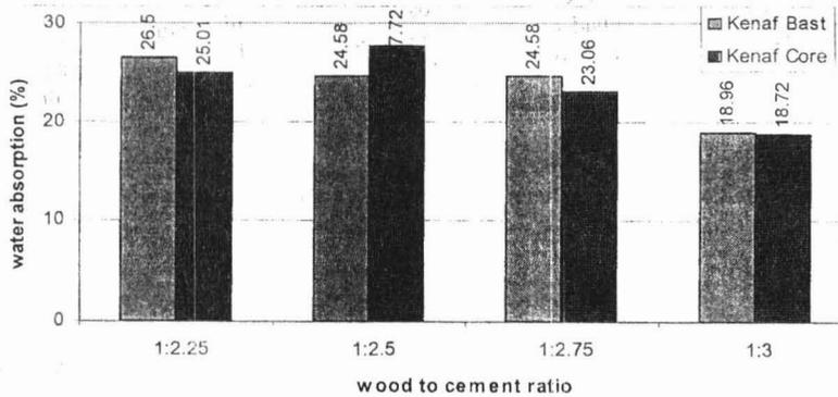
Figure 4: water absorption percentage of kenaf based cement bonded particleboard
