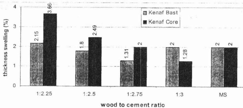
Figure 5: thickness swelling percentage of kenaf based cement bonded particleboard
