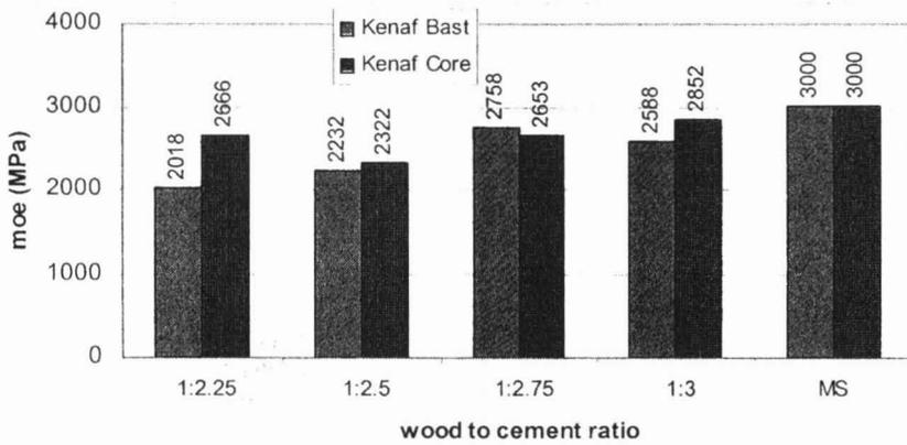
Figure 2: moe value of kenaf based cement bonded particleboard
