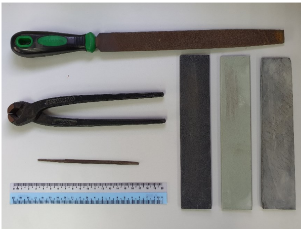
Figure 5: Secondary tools in saring production. From top: Bastard file, pincer, fine file, various grade whetstone. (Source: Author)
