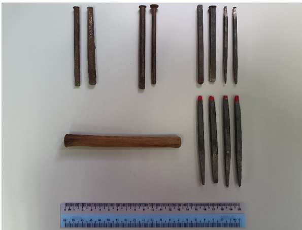
Figure 4: Handmade texturing punches. Top row: Fine line tip makeshift from tile chisel (left), broad line tip makeshift from the concrete nail (middle), and various tips made from steel blanks (right). Bottom row: shaping wooden punch (left) and various steel blanks (right). (Source: Author)
