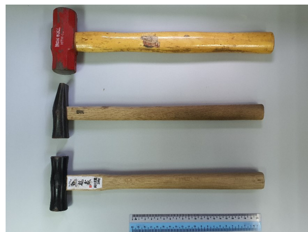
Figure 2: General shaping hammers used in saring production. Sledgehammer (top), Karakami (middle), and Genno (bottom). (Source: Author)
