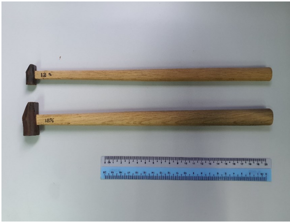
Figure 3: The chasing hammers ( Otafuku ) used during saring bracelet production. (Source: Author)
