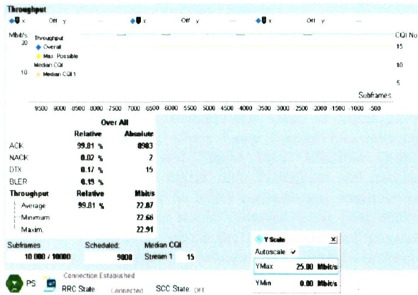
Fig. 14: Transmit Diversity Throughput Measurement Result
